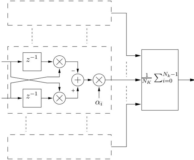
**Figure 3: Architecture of the multicarrier timing offset estimator**
