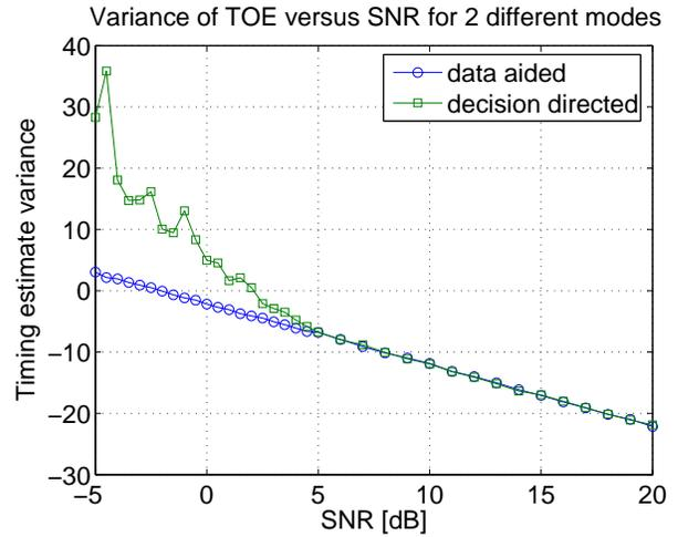
**Figure 8: Variance of timing offset estimate versus SNR for data-aided and decision directed modes. The system uses a 16-point transform WPM based on Daubechies order 6 wavelet.**
