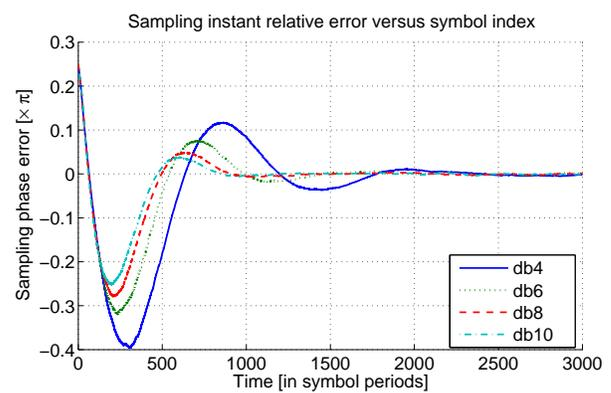
**Figure 6: Comparison of sampling phase acquisition time as a function of the wavelet packet length within the Daubechies family. The modulation is 64-point WPM, the SNR is 20 dB, all the subcarriers are used for timing estimation, and the loop gains are  $\Gamma_{phase} = 2^{-8}$  and  $\Gamma_{period} = 2^{-16}$ . The initial normalised phase error was set to 0.25.**
