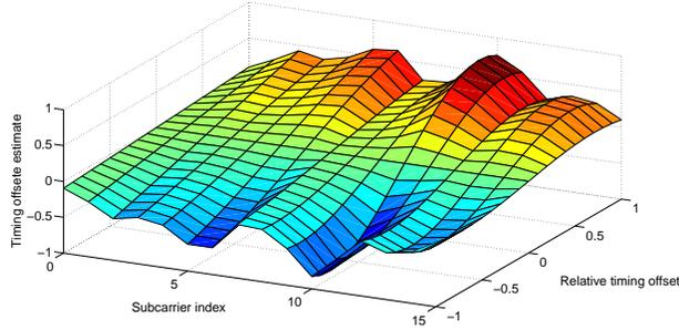
**Figure 1: Estimate of timing offset estimate versus actual timing offset for all subcarriers of a 16-point WPM transform WPM signal using Daubechies order 6 wavelet.**
