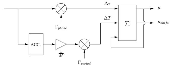
**Figure 4: Architecture of the resampler control block**
