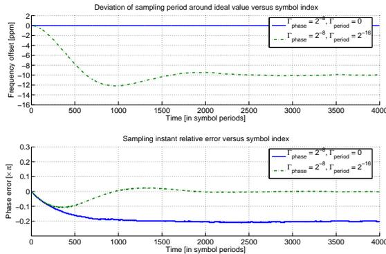
**Figure 5: Algorithm performance comparison without and with sampling period estimation. The modulation is 64-point WPM with Daubechies order 6 wavelet. All the subcarriers are used for timing estimation, and the loop gains are  $\Gamma_{phase} = 2^{-8}$  and  $\Gamma_{period} = 2^{-16}$ .**
