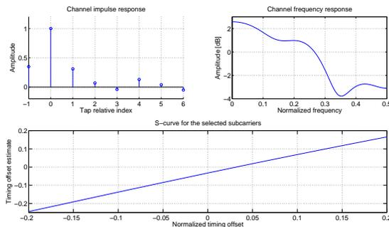
**Figure 7: Overall timing offset estimate versus actual timing offset (S-curve) in presence of a multipath static channel. The channel impulse and frequency responses are plotted in the upper part. The system uses a 16-point transform WPM based on Daubechies order 6 wavelet.**
