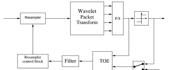
**Figure 2: Architecture of the whole digital symbol synchronisation system**
