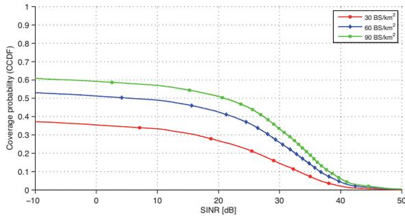
Fig. 3. Coverage probability vs. SINR for different BS densities (mixed materials,  $10^\circ$  beamwidth, PPP BS distribution).
