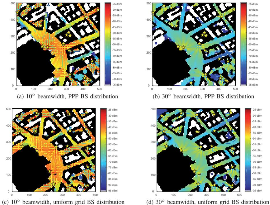
Fig. 7. Heatmap of RSS (dBm) for the uniform grid BS deployment and an example PPP BS deployment, for different antenna beamwidths (90 BS/km<sup>2</sup>, mixed materials). Buildings are shown in black and BS locations as yellow stars; a receiver located in the coloured areas obtains the corresponding RSS from its serving BS, whereas white indicates areas where RSS is below -95 dBm.
