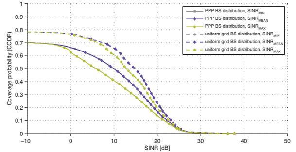
Fig. 2. Coverage probability vs. SINR for the different directional interference models in (4)-(6) (90 BS/km<sup>2</sup>, 30° beamwidth, glass).
