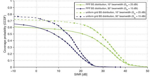
Fig. 6. Coverage probability vs. SINR for different antenna beamwidths and BS distributions (90 BS/km<sup>2</sup>, mixed materials).
