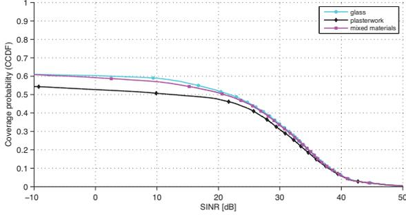
Fig. 5. Coverage probability vs. SINR for different building materials (90 BS/km<sup>2</sup>, 10° beamwidth, PPP BS distribution).
