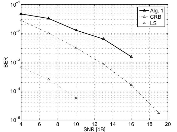
Fig. 5. BER versus SNR. The number of users  $R$  and the number of antennas  $I$  are equal to 4. The spreading gain  $J = 9$ . The frame length is 50 symbols and we assume 3-taps-channels for all users.
