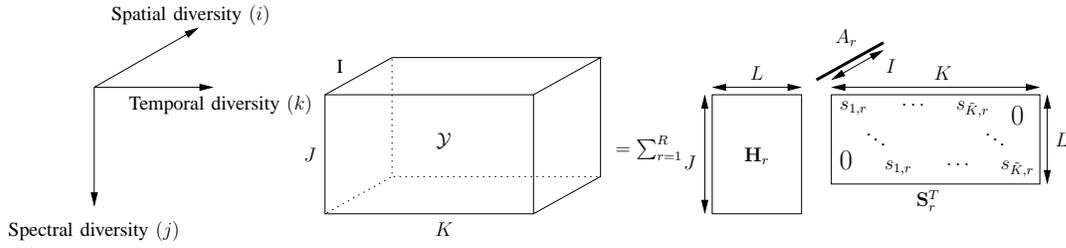
Fig. 2. Decomposition in rank- $(1, L, L)$  terms of the received data tensor.
