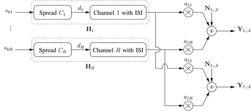
Fig. 1. Discrete-time baseband-equivalent scheme of CDMA transmission.
