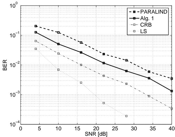
Fig. 3. BER versus SNR. The number of users  $R = 4$ , the spreading code length  $J = 16$  and the number of antennas  $I = 2$ . The frame length is 50 symbols. We assume 2-taps channels for all users.
