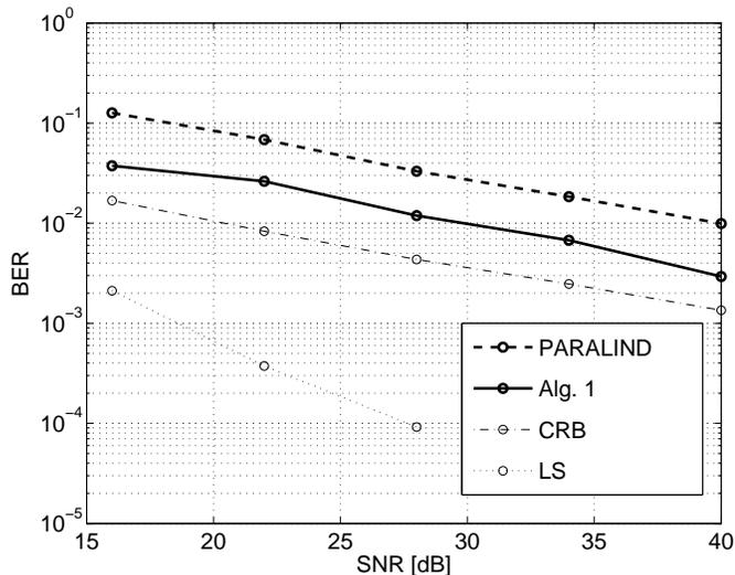
Fig. 4. BER versus SNR. The number of users  $R = 6$ , the spreading code length  $J = 16$  and the number of antennas  $I = 2$ . The frame length is 50 symbols. We assume 2-taps channels for all users.
