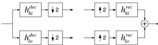
Fig. 2. Wavelet packet elementary block decomposition and reconstruction
