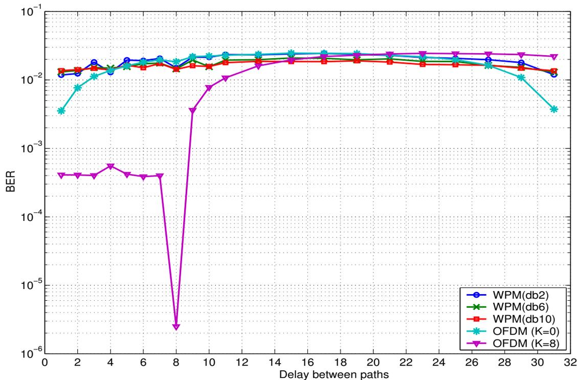
Fig. 5. Performance of WPM versus OFDM in a 2-path time-invariant channel. BER is plotted as a function of the delay of arrival of the second path. The delayed path relative power of  $-3$  dBc and the SNR is 20 dB
