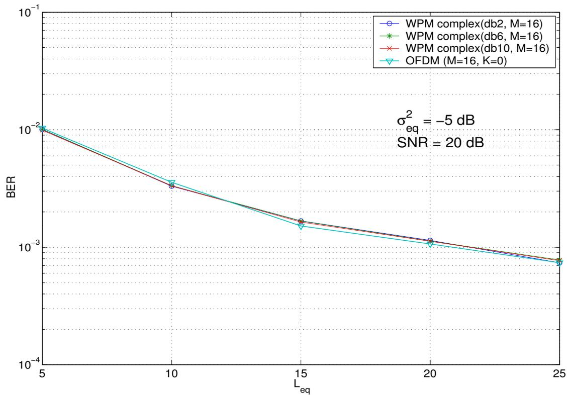
Fig. 6. BER performance of WPM and OFDM schemes with noisy equivalent impulse response, as a function of the length  $L_{eq}$  of imperfectly equalized channel response, at  $\sigma_{eq}^2 = -5$  dB.
