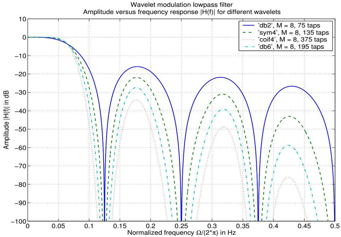
Fig. 4. Frequency domain localization of different wavelets
