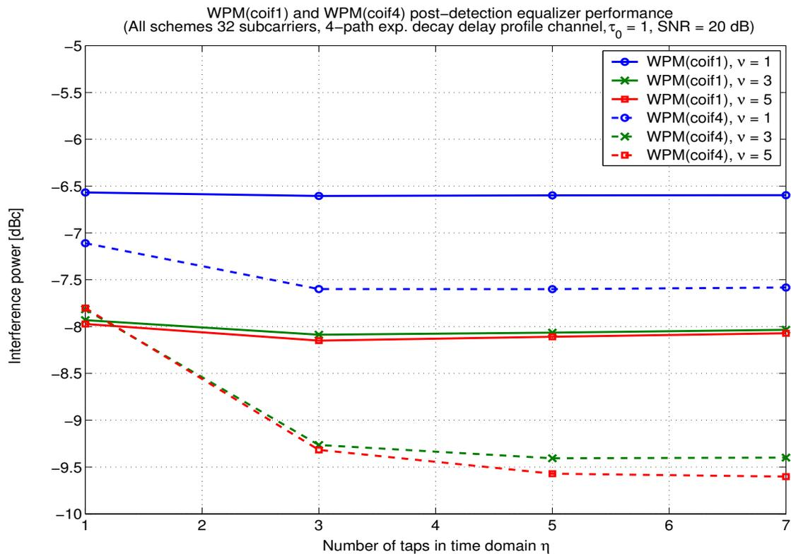
Fig. 7. Comparative performance of WPM(coif1) and WPM(coif4) schemes with post-detection equalization, as a function of the number of equalizer taps  $\eta$  in the time domain and with the number of taps  $\nu$  in the frequency domain as a parameter.
