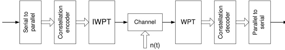
Fig. 1. Wavelet packet modulation functional block diagram
