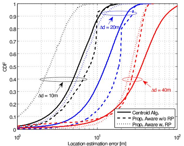
Fig. 2. Cumulative distribution function of the distance between true and estimated location of an AP. Line type determines the reported localization algorithm, line color the grid size of the measurement grid.
