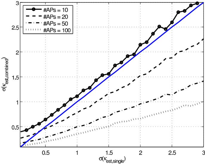
Fig. 5. RMSE of  $\kappa$  estimation: Comparison between RMSE for  $\kappa$  estimation through averaging over the locally estimated values and  $\kappa$  estimation through normalization. With small number of routers the  $\kappa$  estimation error lowers below the compared singular variance, marked by the blue isoperformance line.
