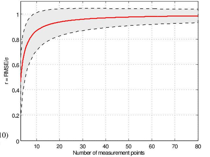
Fig. 3. Ratio of the root mean-square error and the shadowing deviation  $\sigma$  for single AP scenario with known location vs. number of measurement points. The red center line shows the average ratio. The gray area shows the 25<sup>th</sup> and 75<sup>th</sup> percentile after 100,000 simulation runs.
