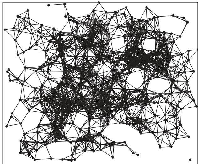
**Figure 5. Ad hoc network topology using the random waypoint model.**
