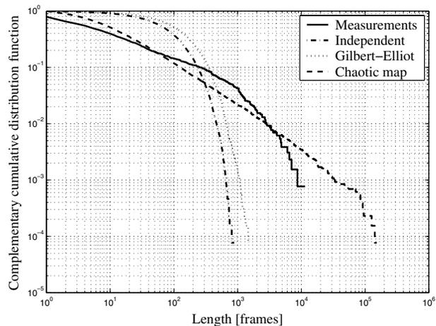
Figure 1. Example for the run length distribution in bad channel conditions.
