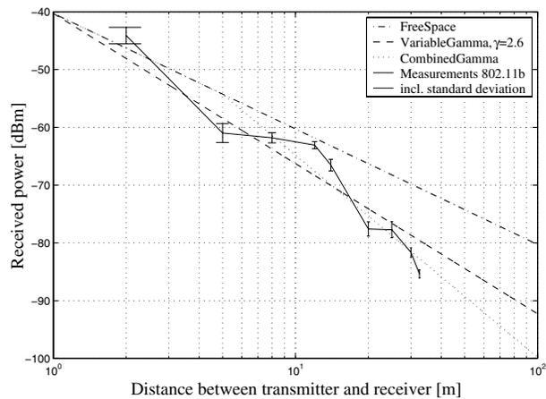
Figure 2. Radio propagation measurements with IEEE 802.11b.
