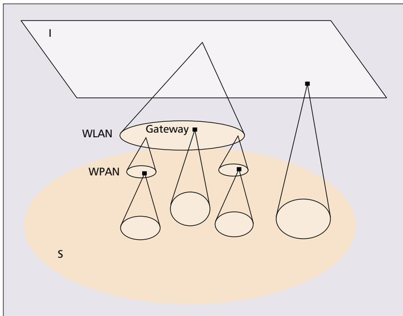
**Figure 1.** The logical architectural relationship between the Internet and sensor domains. Gateways are the key to interconnecting these two. Mobility increases moving from the Internet domain down to the sensor domain.
