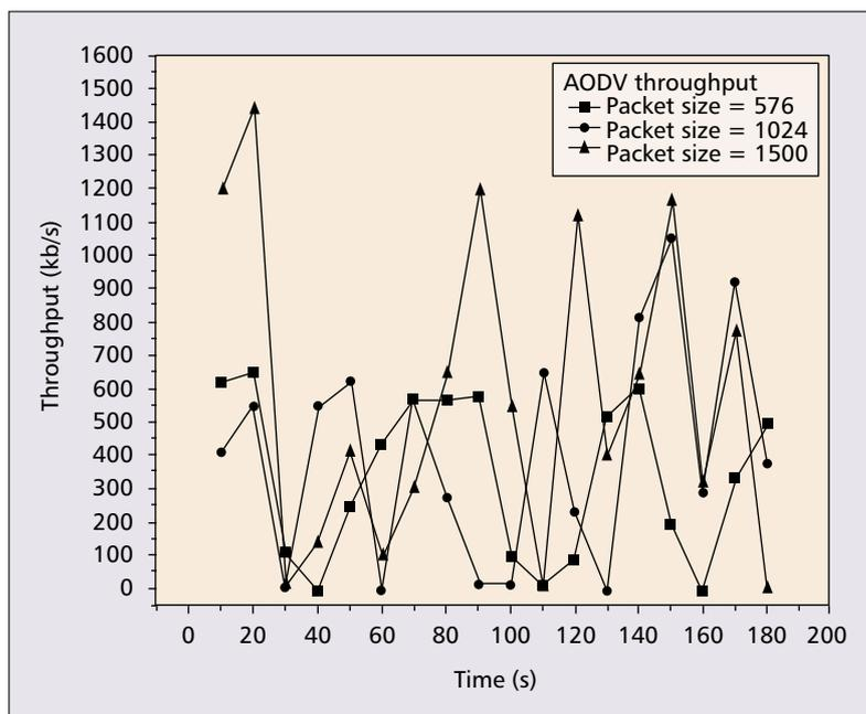
Figure 4. The performance of AODV with TCP over an error-prone three-hop IEEE802.11 link.
