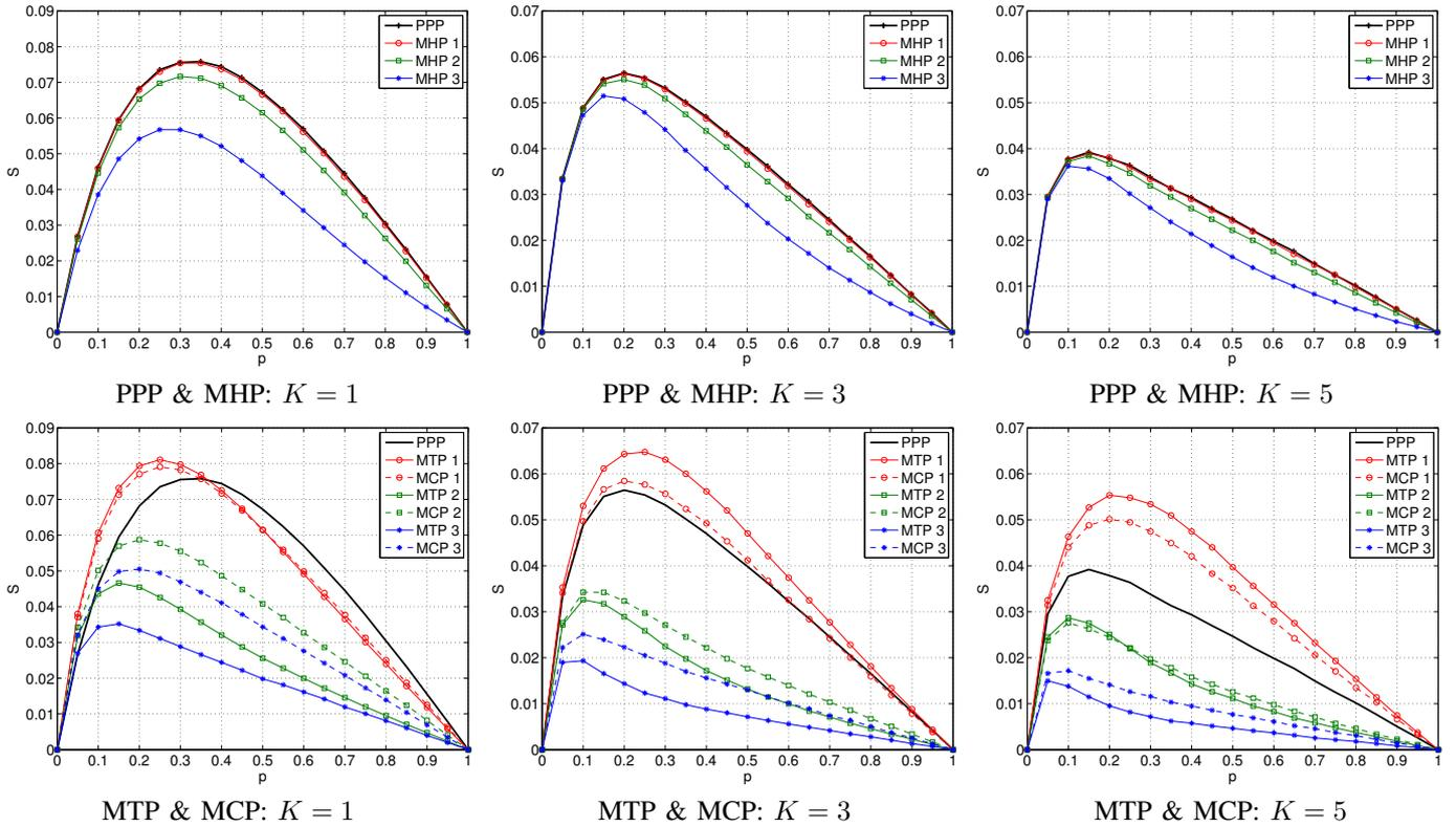
Fig. 2. Local Throughput  $S$  over transmission probability  $p$ . Average number of neighbors of the PPP  $K = 1, 3$ , and  $5$ .  $N = 100$ ,  $\alpha = 4$ , and  $\Theta = 10$  dB. Transmissions over Rayleigh fading channels.
