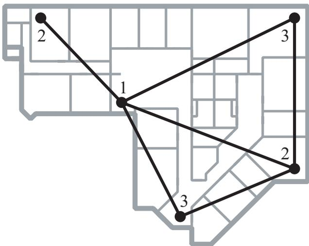
Figure 1: Example interference graph.
