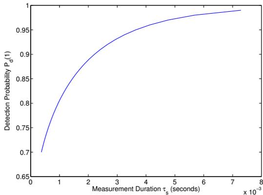
Fig. 3. The relationship between detection probability  $P_d(1)$  and spectrum measurement duration  $\tau_s$ .
