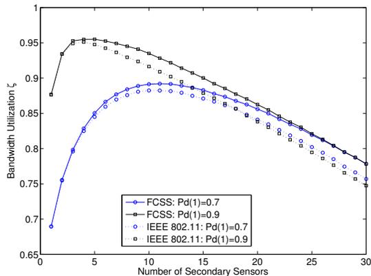
Fig. 6. A comparison between FCSS and the IEEE 802.11 scheme where the sensing and reporting phases are temporally separated.
