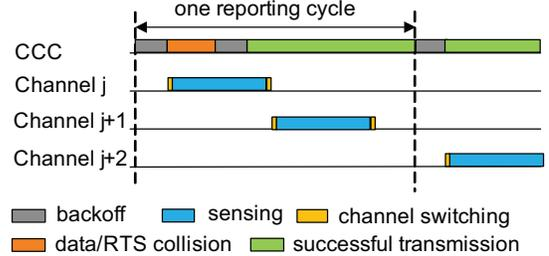
Fig. 2. An illustration of implementation details during  $T_{sr}$ . In the two-way handshake, the length of the collision box approximates that of the successful transmission box.
