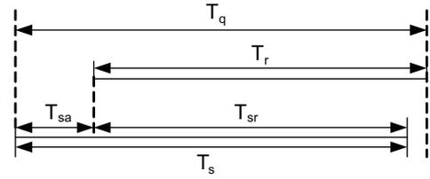
Fig. 1. A quiet period with overlapped sensing and reporting phases
