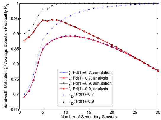
Fig. 4. A comparison of simulation and analytical results. The selection of  $m_{sa}$  meets the condition that each channel is sensed at least once during  $T_{sa}$ .
