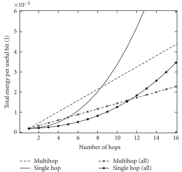
FIGURE 5: Comparison of the node  $n$  only and all node transmission traffic cases. It can be seen that the crossover point is further in the all nodes transmitting case. Node spacing  $d$  is 10 m and the path loss exponent  $\alpha$  is 2.5.
