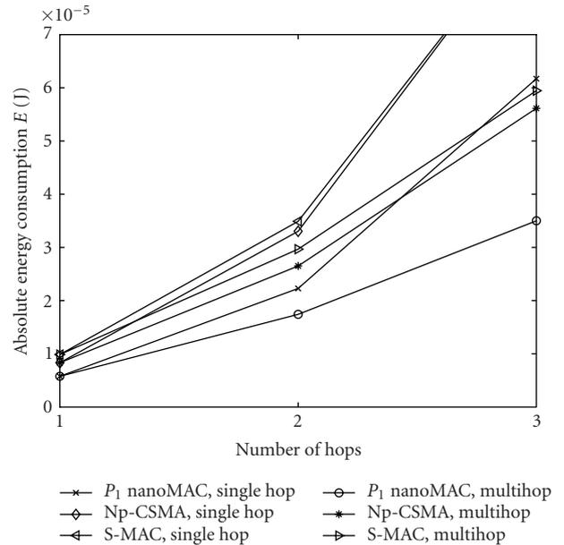
FIGURE 11: Optimal spacing with characteristic distance  $d_{\text{char}}$ . Common sleep group for single-hop versus multihop communications. With  $d_{\text{char}}$ , multihop forwarding always outperforms single-hop communications but, for example, nanoMAC single-hop communications outperform np-CSMA and S-MAC multihop forwarding with 2 hops ( $d = 31.5$  m times multiplier  $N$ , path loss exponent  $\alpha = 2.5$ ).
