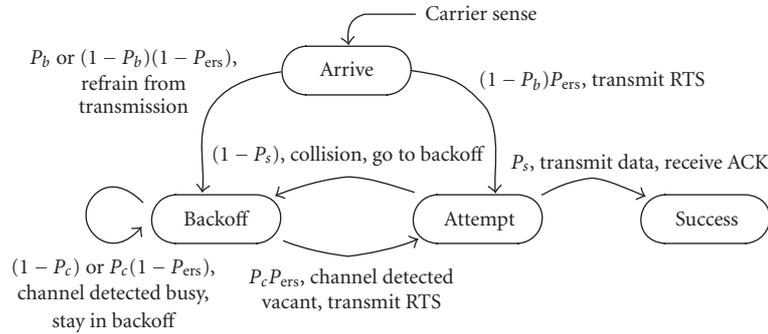
FIGURE 6: Transmit energy model for nanoMAC. The arrows present energy consuming transitions from one state to a new state while the states are instant and do not consume energy.  $P_b$ ,  $P_{ers}$ ,  $P_s$ , and  $P_c$  are transition probabilities.
