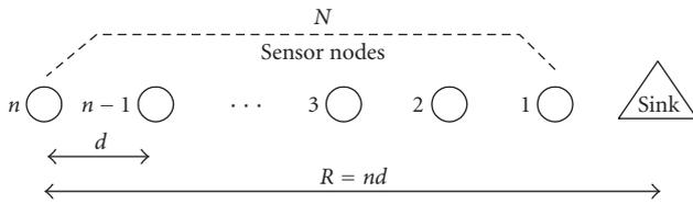
FIGURE 1: A simple linear sensor network of  $N$  nodes. Nodes are separated by distance  $d$  and to reach the sink node, node  $n$ 's packets require  $n$  hops resulting in an overall distance of  $R$ .
