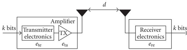
FIGURE 3: Typical narrowband radio energy consumption model where  $k$  bits are transmitted and  $e_{te}$  and  $e_{ta}$  are the transmitter electronics and amplifier energy consumption per bit, respectively. The transmission distance is  $d$  and the  $k$  bits are received by the receiver electronics consuming  $e_{rx}$  energy per bit.
