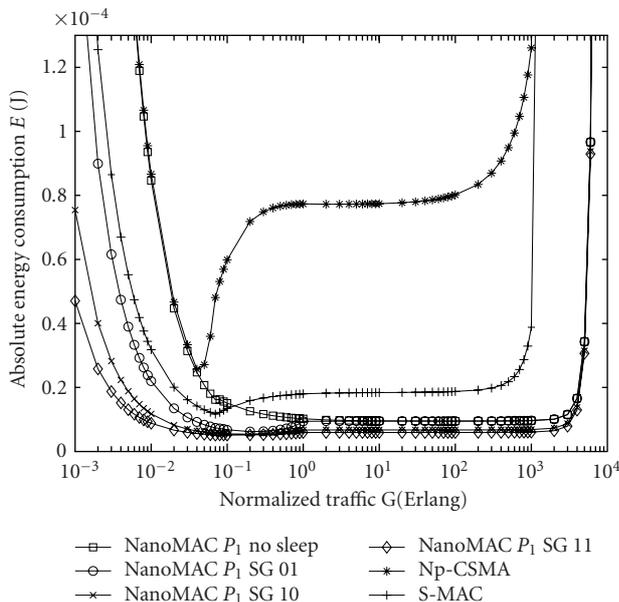
FIGURE 9: Energy consumption of nanoMAC with sleep groups, np-CSMA, and S-MAC per transmitted MSDU bit in the worst-case scenario with respect to  $G$ . A node transmits as often as possible with a 10% duty-cycle constraint and is the recipient for all the other transmissions in the channel.
