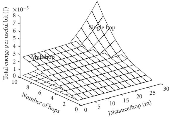
FIGURE 4: Total energy for the node  $n$  transmitting case. This plot shows the relationship between multihop and single-hop energy efficiency. Single hop is typically more efficient within the radio's transmission range. The path loss exponent  $\alpha$  is 2.3 in this case.
