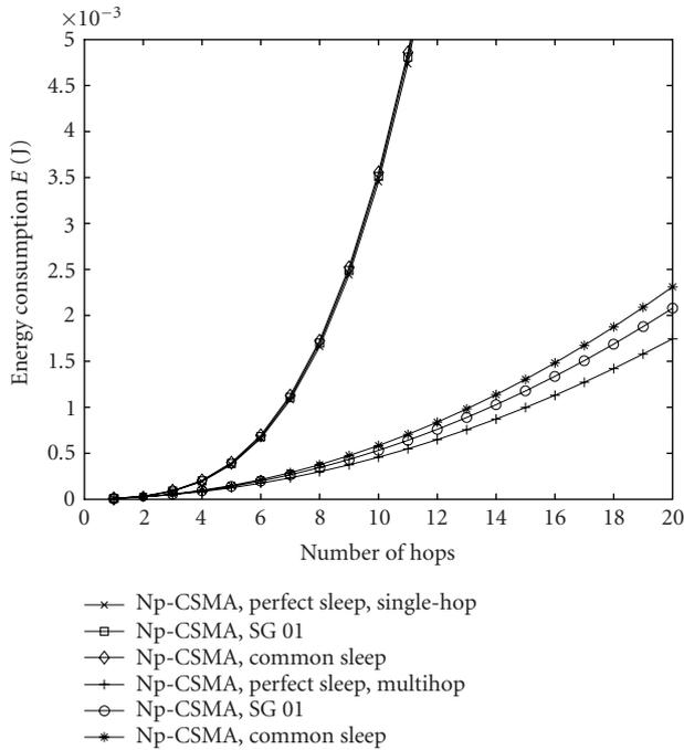
FIGURE 10: Nonpersistent CSMA with a linear topology. Comparison of single-hop versus multihop communications with characteristic distance  $d_{\text{char}}$ . All nodes are transmitting and different sleep groups are utilized ( $d = 31.5$  m times multiplier  $N$ , path loss exponent  $\alpha = 2.5$ ).
