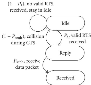
FIGURE 7: The receive energy model for nanoMAC. The arrows present energy consuming transitions from one state to a new state while the states are instant and do not consume energy. *Idle* is the entry point to the system and no energy is consumed before a transmission by another device is attempted.  $P_s$  and  $P_{senh}$  are transition probabilities.
