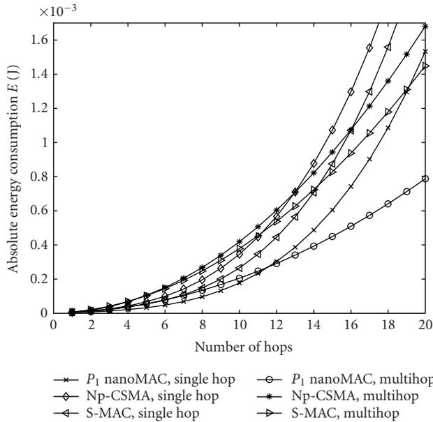
FIGURE 12: Np-CSMA, S-MAC, and nanoMAC energy consumption with nonoptimal spacing of  $d = 10$  meters. Common sleep group applied for all the protocols comparing single-hop versus multihop communications. All the protocols' curves cross implying single-hop communications outperform multihop communications up to the crossover point ( $d = 10$  m times multiplier  $N$ , path loss exponent  $\alpha = 2.5$ ).
