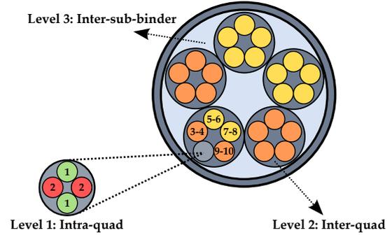
Fig. 1. 50-pair cable binder layout and inter-pair relationships. Hierarchical levels (intra-quad, inter-quad and inter-sub-binder) are indicated by arrows, whereas relative pair positions (near/far-neighbors) are denoted by different colors. If pair 1 is evaluated, red, orange and yellow pairs correspond to intra-quad, near- and far-neighbors, respectively.
