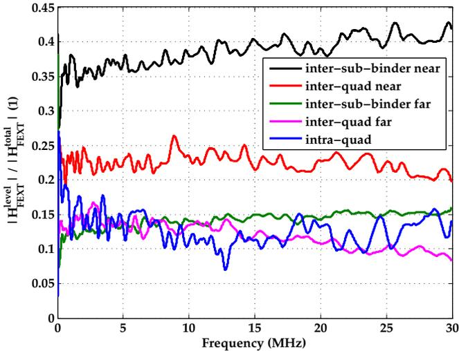
Fig. 3. Mean FEXT magnitude fraction of inter-pair relationships in a fully-occupied 50-pair binder. Inter-sub-binder and inter-quad near-neighbors concentrate about 60% of the interference magnitude.
