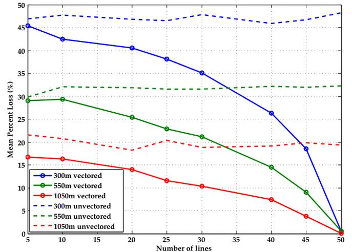
Fig. 5. Vectored and non-vectored systems performance for different number of controlled lines. The difference between dashed and solid curves is the gain obtained by vectoring in terms of the proximity to the FEXT-free performance.
