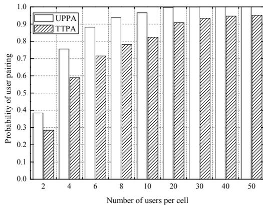
Fig. 4. Probabilities of user pairing with different power allocation schemes.
