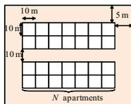
Fig. 2. Bird's-eye view of the urban building block model (each building of  $N$  apartments per row has  $L$  floors) [10].  $N$  is randomly varied between 5 and 10, and  $L$  between 3 and 5, with a 3 m height per floor.
