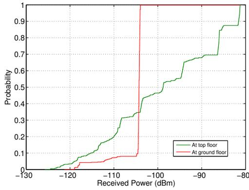
Fig. 8. Received power at the ground floor and at a top floor for a building from a neighboring cochannel MBS.
