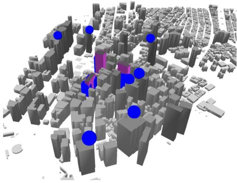
Fig. 1. An illustration of the 3D building data set used in the study, with high risers used for femtocell deployments shown in purple, and macrocellular antenna sites shown in blue.
