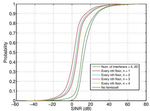
Fig. 6. Impact of density of FAP deployment in surrounding interferers, for FAP to MUE interference.
