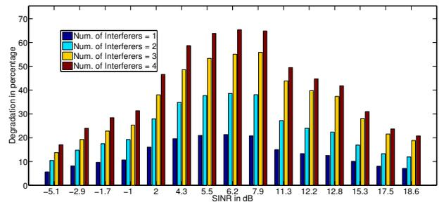
Fig. 7. Impact of number of surrounding interferers for FAP to MUE interference.
