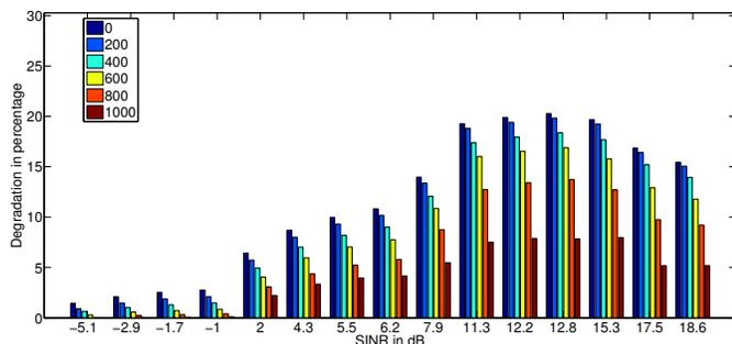
Fig. 5. Impact of FFR as a function of the frequency reuse radius in meters for bandwidth of 1.4 MHz. Radius of zero refers to the case of no FFR being used.
