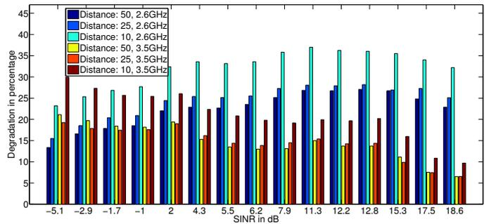
Fig. 11. Degradation charts for normalized CDFs for 2.6 GHz and 3.5 GHz bands. Degradation is computed compared to the case of no interferers.
