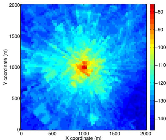
Fig. 1. RSCP coverage map measured in dBm used as the ground-truth.
