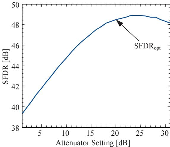
Fig. 4. Spurious Free Dynamic Range over Attenuator sweep
