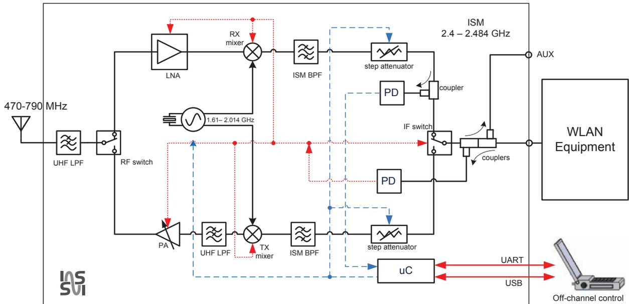
Fig. 1. Complete block diagram of the proposed white space converter.
