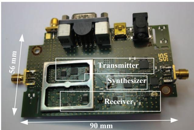
Fig. 5. Hardware of the white space converter prototype
