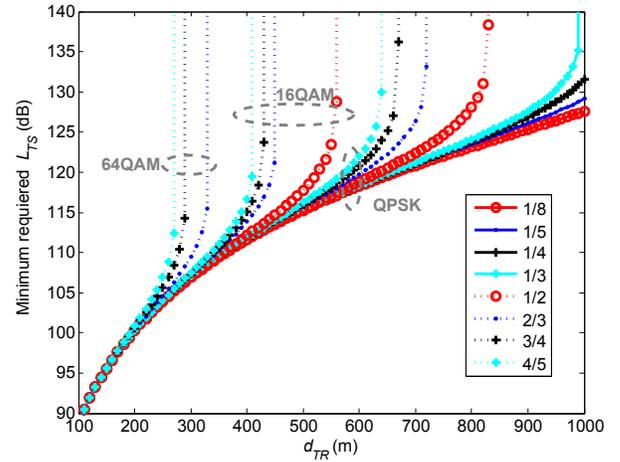
Fig. 2. Minimum required  $L_{TS}$  as a function of  $d_{TR}$  for different services (The labels represent the different coding rates).
