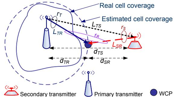
Fig. 1. The considered model for evaluating the impact of correlation ( $L$ ,  $d$  and  $r$  represent the path loss, distance and shadowing factor correlation, respectively. Subscripts  $T$ ,  $R$  and  $S$  represent the primary transmitter, the primary receiver and the secondary transmitter, respectively. WCP stands for Worst Case Position of primary receivers).
