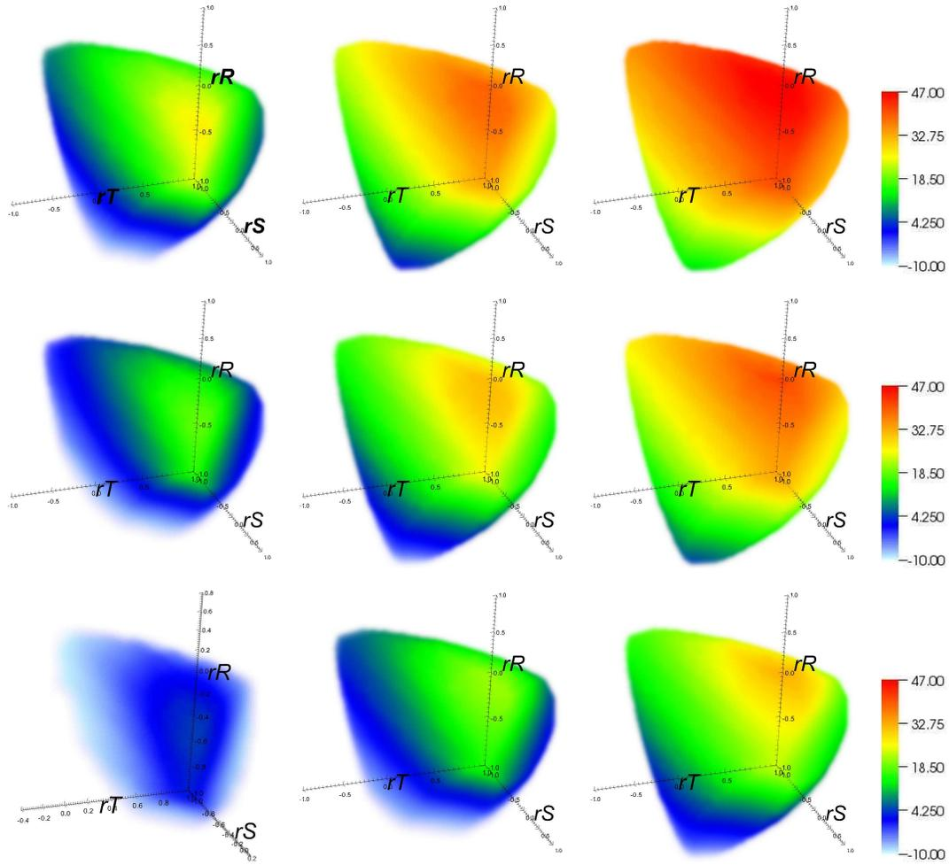
Fig. 3. The values of  $P_S$  in dBW as a function of the correlation coefficients for  $d_{TR} = 500$  m. The different columns represent different values of  $L_{TS}$  (i.e., 121 dB, 127 dB and 133 dB from left to right) and the different rows represent different  $\gamma_r$  (i.e., -2.6 dB, 4.5 dB and 10.9 dB from top to bottom). The values of  $\gamma_r$  correspond to pairs (modulation, coding rate) that are respectively (QPSK, 1/8), (QPSK, 1/2) and (16QAM, 1/2) [19].
