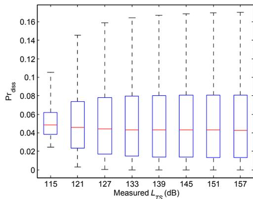
Fig. 4. The box plots of  $\text{Pr}_{\text{diss}}$  for  $\gamma_r = -2.6$  dB. Each box plot represents the distribution of  $\text{Pr}_{\text{diss}}$  for a given  $L_{TS}$  when  $P_S$  is computed assuming that there is no shadowing correlation, whereas the latter varies in the interval  $[-1, 1]$  (the central mark is the median, the edges of the box are the 25th and 75th percentiles, and the whiskers extend to the maximum and minimum).
