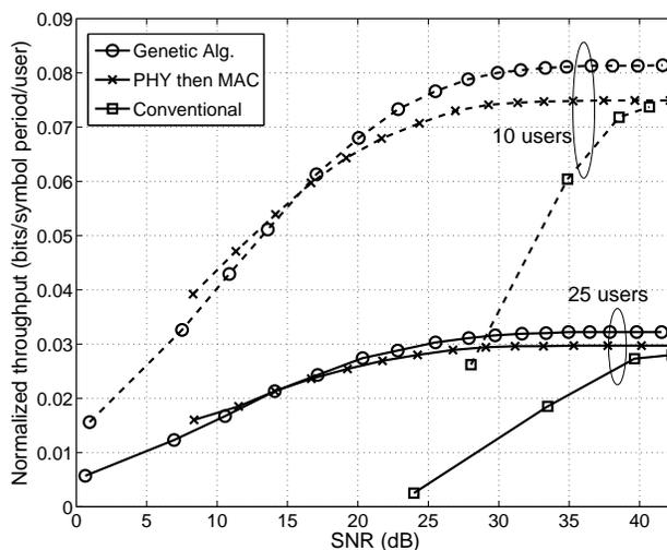
Fig. 6. Cross-Layer Optimization for OFDM-based CSMA/CA system: Joint Power Optimization / Bit-loading Algorithm / Minimum Contention Window Size / Maximum Backoff Stage. Target  $PER^* = 10^{-3}$ .
