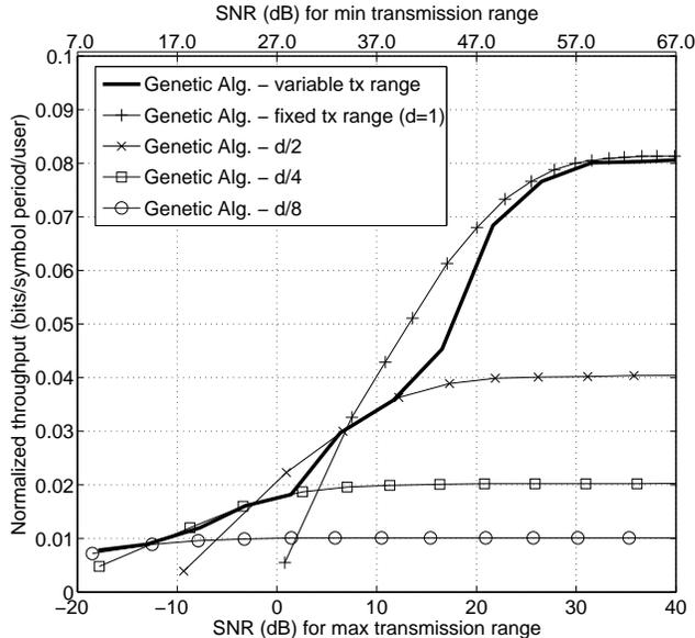
Fig. 8. Cross-Layer Optimization for OFDM-based CSMA/CA system with multihop transmission: Joint Power Optimization / Bit-loading Algorithm / Minimum Contention Window Size / Maximum Backoff Stage / Variable Range. Target  $PER^* = 10^{-3}$ . System load = 10.
