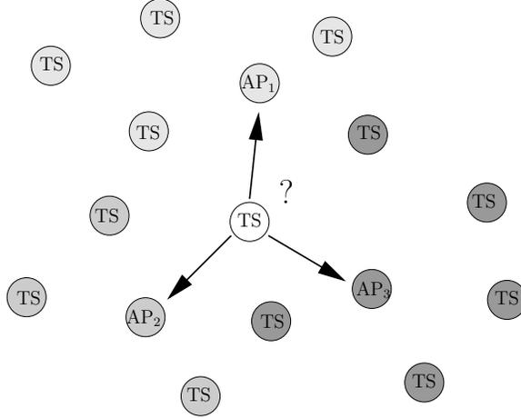
Fig. 9. System model in Scenario 4: A newcomers terminal station seeks to establish connection with one of the access points  $AP_1$ ,  $AP_2$  and  $AP_3$  that are within its transmission range. Each transmission link from  $TS$  to  $AP_i$ ,  $i \in \{1, 2, 3\}$  is modeled as having additive white Gaussian noise with flat fading coefficient  $a_i$ . In this example, the current load is 4 for  $AP_1$ , 3 for  $AP_2$  and 5 for  $AP_3$ .
