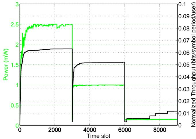
Fig. 11. Power adaptation in OFDM-based CSMA/CA system with decreasing power constraints: Start with full power utilization (Target POWER = 2.50 mW) for the first 3000 time slots, then switch to 1 mW mode for the next 3K time slots, then lower power (0.15 mW). Target PER\* =  $10^{-3}$ . Network load = 10.
