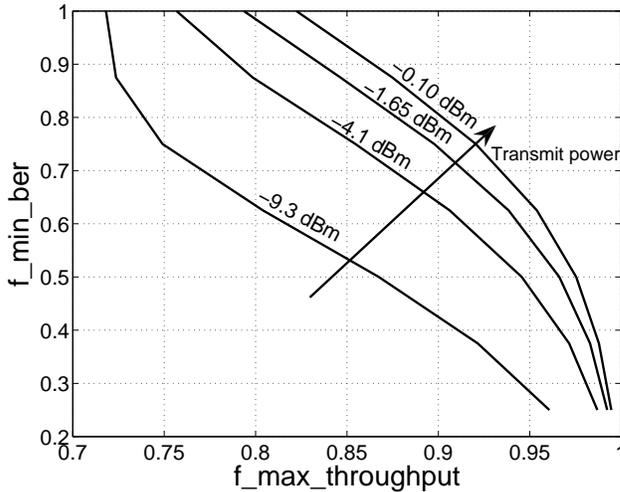
Fig. 3. Search direction example. Both objectives  $f_{\max\_throughput}$  (2b) and  $f_{\max\_ber}$  (3b) conflict with each other for any transmission power.
