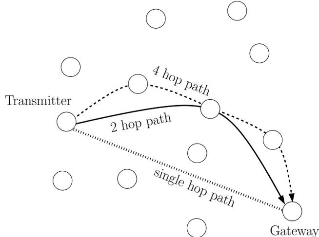
Fig. 7. System model for Scenario 3: Variable range routing for multihop transmission in a wireless mesh network. A transmitter transmits data to the gateway node via multihop transmission. There are several possible paths. Dotted line: direct transmission; solid line: 2-hop transmission; dashed line: minimum transmission range.
