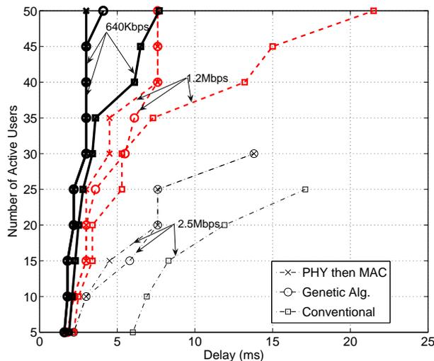
Fig. 12. Maximum number of active users in the network with respect to the delay bound. Target packet error rate of 2% in OFDM-based CSMA/CA system for high data rate streaming transmission (video).
