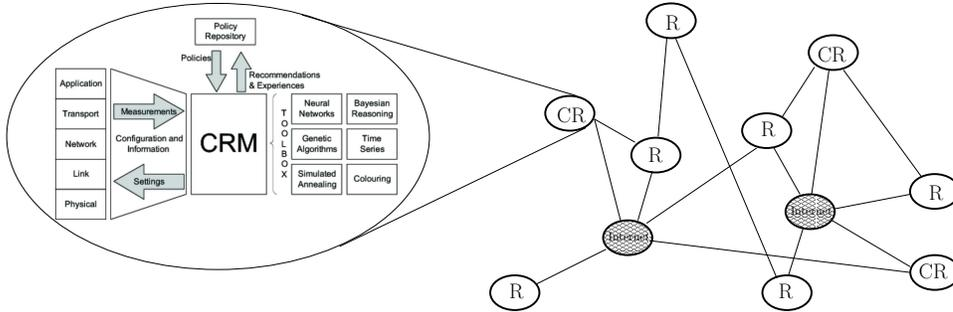
Fig. 1. Functional architecture of the Cognitive Radio Manager with the interfaces to different entities.
