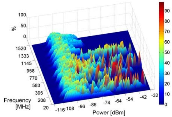
Fig. 13. Amplitude probability distribution of the power levels measured during the outdoor campaign from 05-Feb-2007 11:13:52 to 12-Feb-2007 09:06:42 in the spectrum band 20-1520 MHz.
