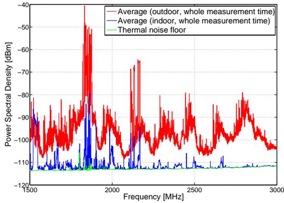
Fig. 11. Comparison of indoor and outdoor measurement results to the measured thermal noise floor for 1500 to 3000 MHz.
