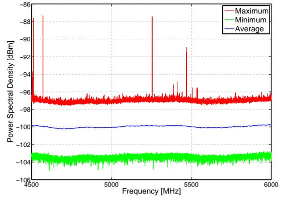
Fig. 9. Minimum, average and maximum PSD measured at the outdoor location in the spectrum band 4 from 4500-6000 MHz.
