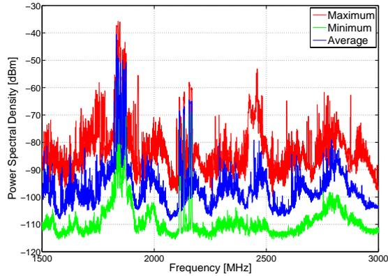
Fig. 7. Minimum, average and maximum PSD measured at the outdoor location in the spectrum band 2 from 1500-3000 MHz.
