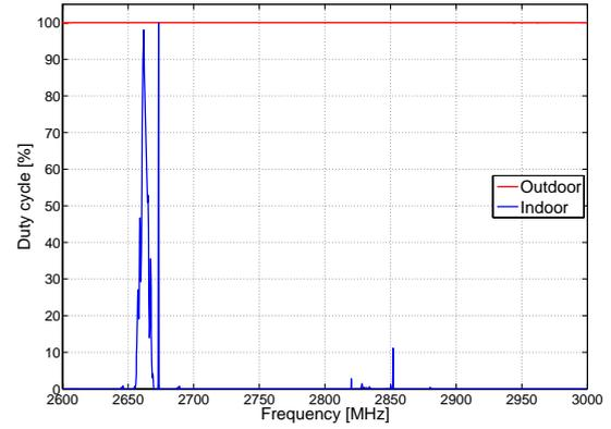
Fig. 12. Comparison of duty cycle based on indoor and outdoor measurement for 2600 to 3000 MHz.
