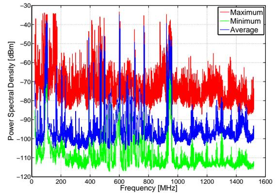
Fig. 6. Minimum, average and maximum PSD measured at the outdoor location in the spectrum band 1 from 20-1520 MHz.
