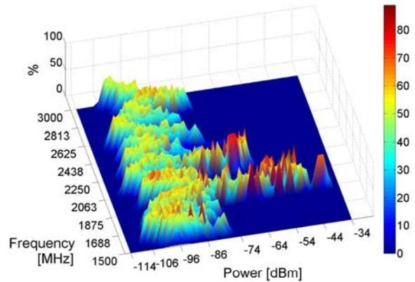
Fig. 14. Amplitude probability distribution of the power levels measured during the outdoor campaign from 12-Feb-2007 09:47:42 to 20-Feb-2007 08:47:28 in the spectrum band 1500-3000 MHz.
