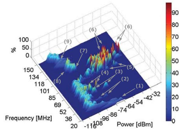
Fig. 15. Amplitude probability distribution of the power levels measured during the outdoor campaign in the spectrum band 20-150 MHz with more details and marks.
