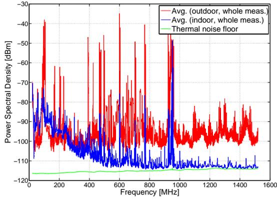
Fig. 10. Comparison of indoor and outdoor measurement results to the measured thermal noise floor for 20 to 1520 MHz.
