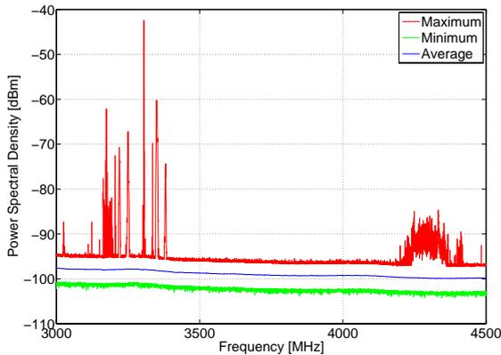
Fig. 8. Minimum, average and maximum PSD measured at the outdoor location in the spectrum band 3 from 3000-4500 MHz.
