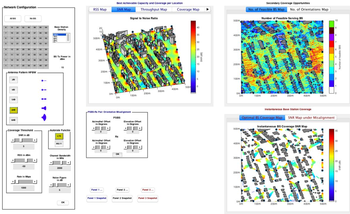
Fig. 1. Planning tool GUI, illustrating different coverage and robustness metrics to characterize mm-wave network performance.
