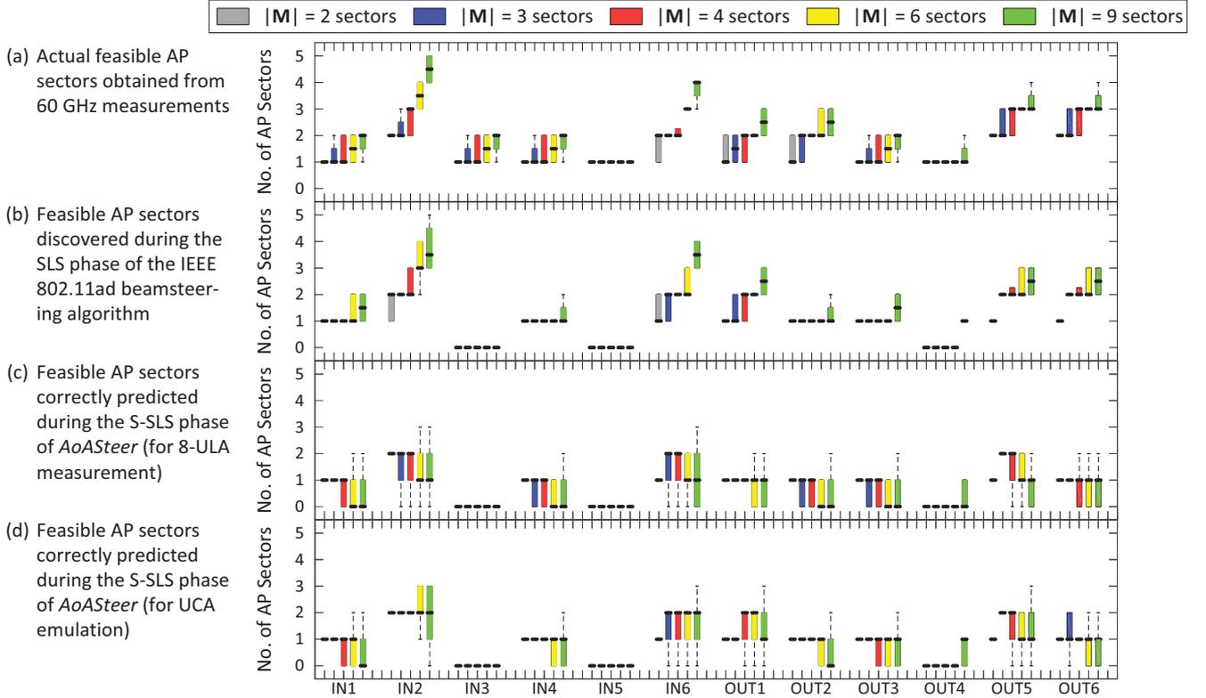
Fig. 8: Actual feasible AP sectors, feasible AP sectors discoverable by the IEEE 802.11ad beamsteering algorithm and feasible AP sectors correctly predicted by our 2.4 GHz AoA estimation system for different locations (cf. Table II) and values of  $|M|$ .
