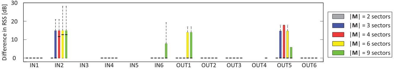
Fig. 11: Difference in RSS at the UE for the links established via *AoASteer* (number of estimated AP sectors,  $|\mathbf{m}| = 3$ ) and the IEEE 802.11ad beamsteering algorithm for different locations (cf. Table II) and number of antenna sectors per node,  $|\mathbf{M}|$ .
