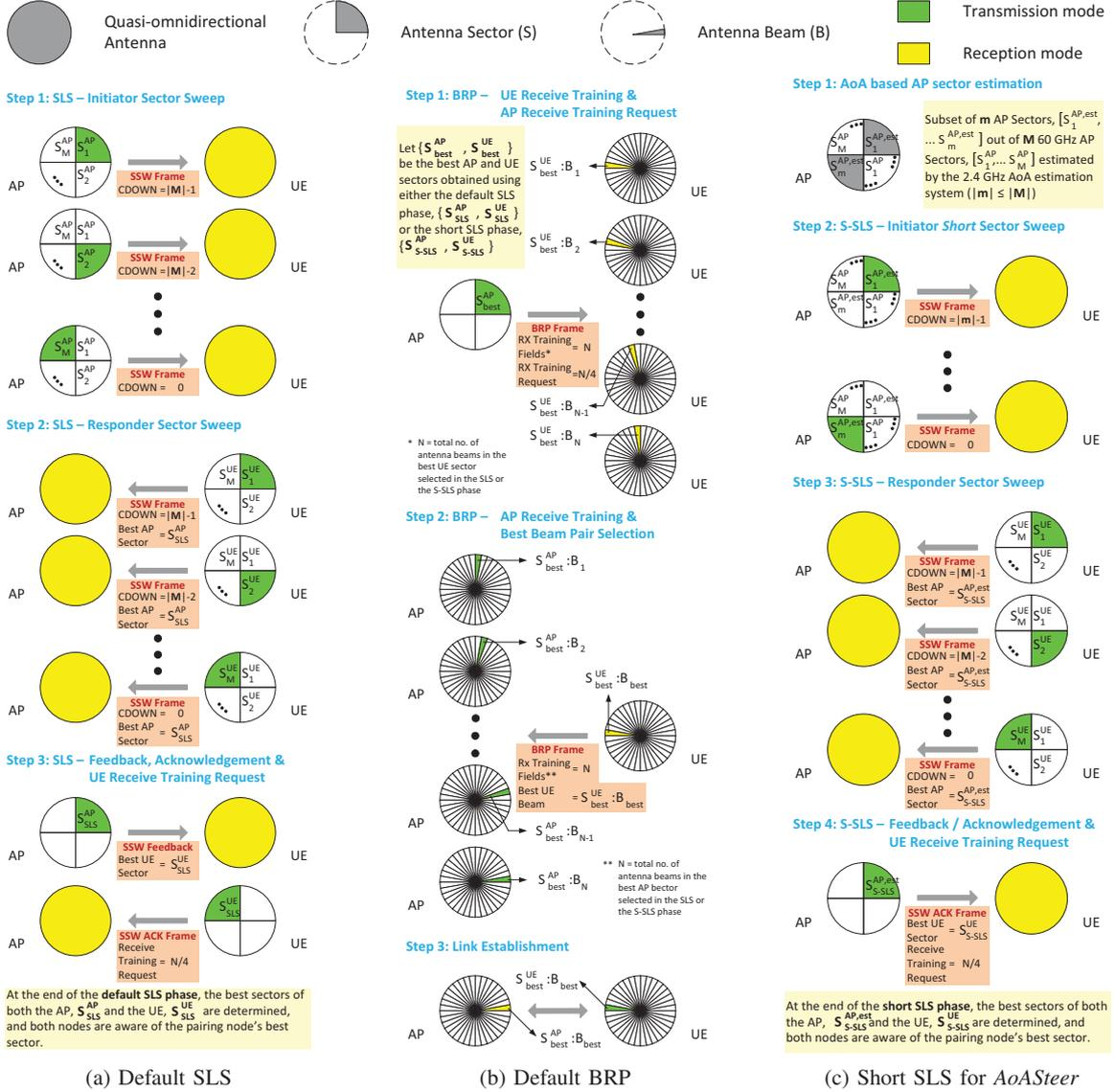
Fig. 1: Example Sector Level Sweep (SLS) and Beam Refinement Phase (BRP) operations for the default IEEE 802.11ad beamsteering algorithm and the proposed Short Sector Level Sweep (S-SLS) phase operations for AoASteer.
