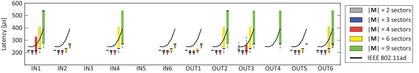
Fig. 10: Link establishment latency using *AoASteer* (number of estimated AP sectors,  $|\mathbf{m}| = 3$ ) for different locations (cf. Table II) and number of antenna sectors per node,  $|\mathbf{M}|$ . An emulated UCA is employed for 2.4 GHz AoA estimation.
