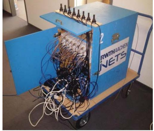
Fig. 7: 2.4 GHz AoA estimation system receiver setup consisting of 8-element uniform linear array (8-ULA) antenna.
