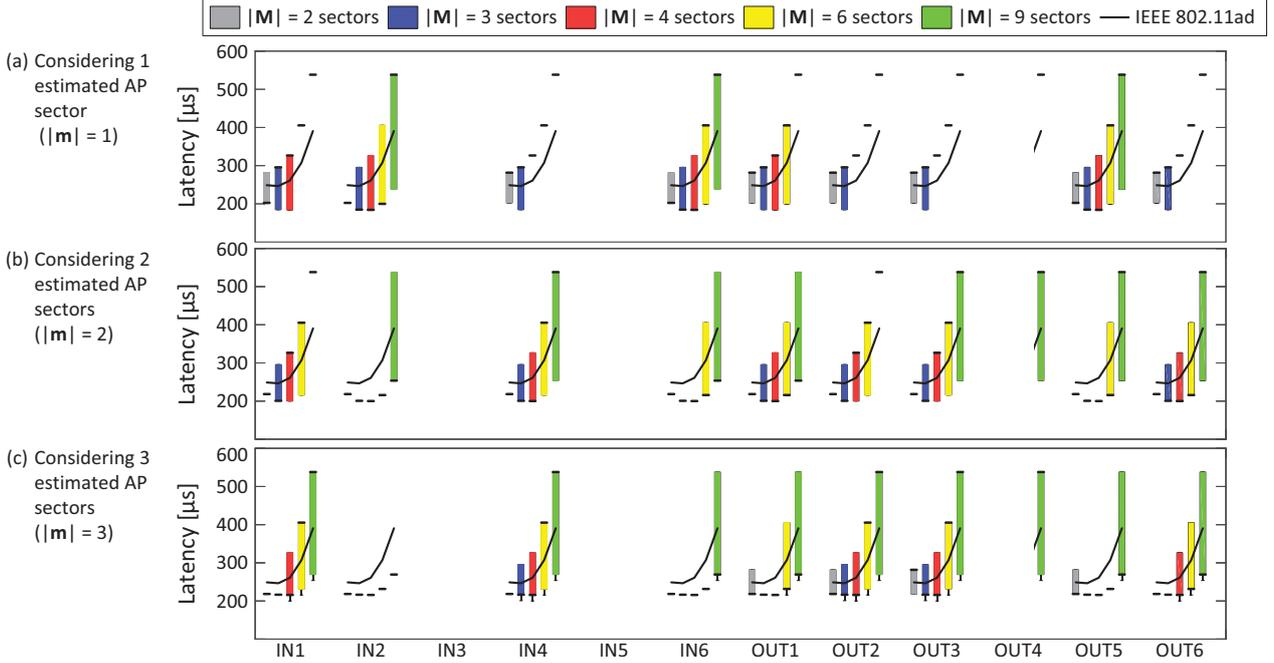
Fig. 9: Link establishment latency using *AoASteer* for different locations (cf. Table II), number of estimated AP sectors,  $|\mathbf{m}|$  and number of antenna sectors per node,  $|\mathbf{M}|$ .
