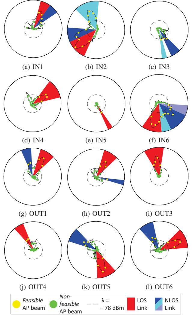
Fig. 5: Polar plot for RSS along different AP beams for the different locations. AP beams corresponding to the same feasible LOS/NLOS link (cf. Figs.3 and 4) are grouped together by background color.
