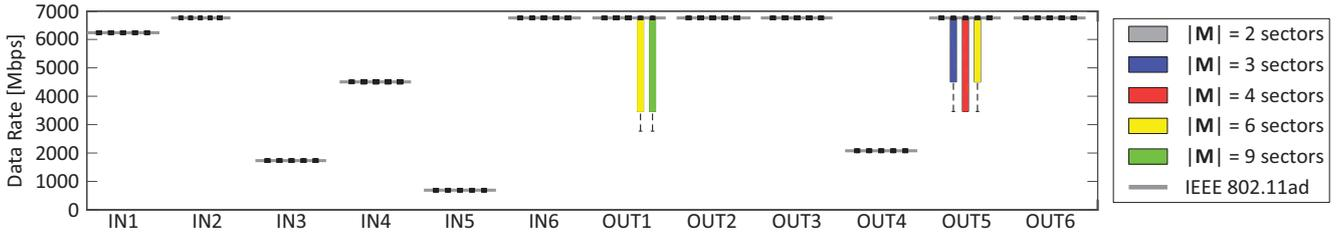
Fig. 12: Data rate achieved for the links established using *AoASteer* (number of estimated AP sectors,  $|\mathbf{m}| = 3$ ) for different locations (cf. Table II) and number of antenna sectors per node,  $|\mathbf{M}|$ .
