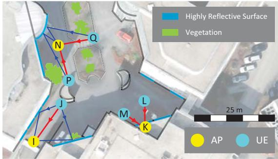
Fig. 4: Outdoor measurement locations showing the 60 GHz AP-UE links (LOS links: red; NLOS links: blue).
