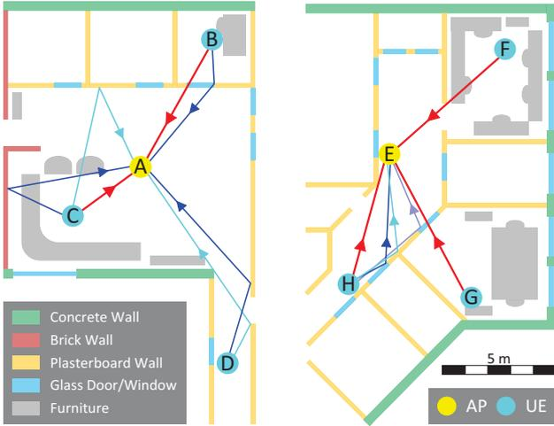
Fig. 3: Indoor measurement locations showing the 60 GHz AP-UE links (LOS links: red; NLOS links: blue).
