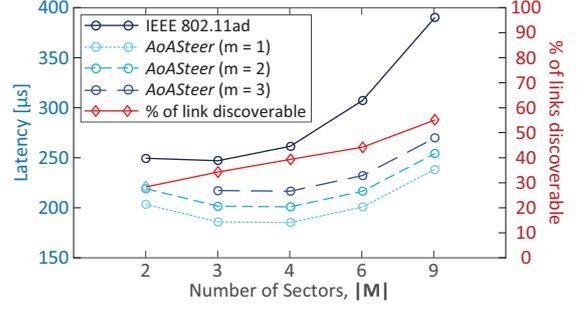
Fig. 2: Link establishment latency for *AoASteer* (best-case) and the IEEE 802.11ad beamsteering algorithm, and the percentage of feasible links discoverable for different number of antenna sectors.
