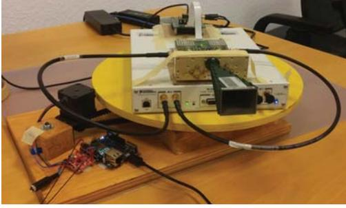
Fig. 6: 60 GHz USRP-SiversIMA transceiver with  $10^\circ$  beamwidth fixed beam horn antenna on a turntable.
