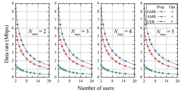
Fig. 2. Comparison of the throughput performance of the proposed scheme with the optimal value.
