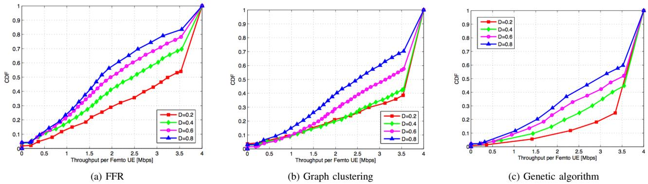
Fig. 7. Distribution of femtocell downlink throughput for different frequency assignment algorithms and deployment ratios.
