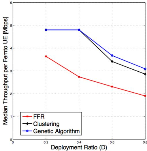
Fig. 6. Median femto UE throughput as a function of the deployment ratio.
