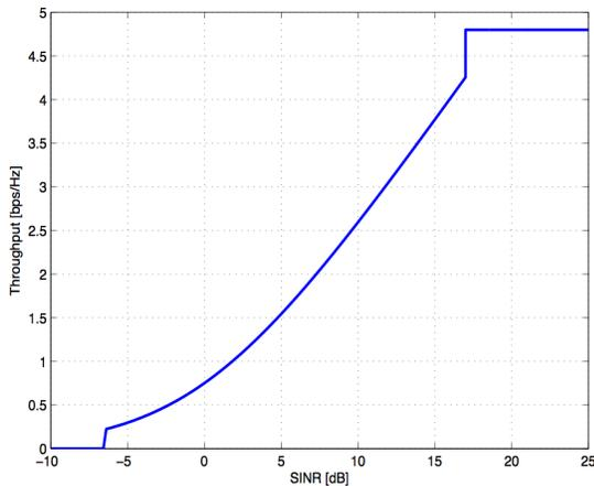
Fig. 3. Truncated Shannon capacity law used to estimated LTE downlink throughput based on the SINR of a resource block.
