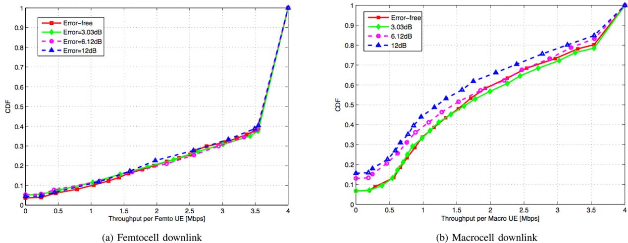
Fig. 8. Distribution of femtocell and macrocell downlink throughputs for the clustering method in the presence of estimation errors for link gains.
