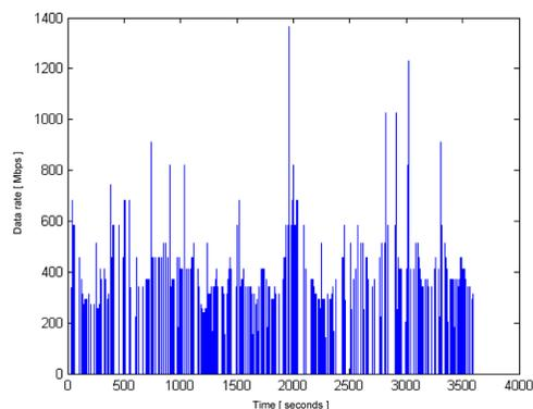
Fig. 3. Example throughput achieved using LMDS / 60 GHz hotspots.
