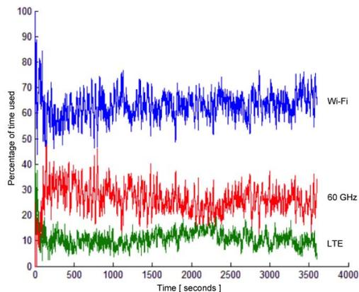
Fig. 2. Percentage of time given radio technology is used in the simulation.
